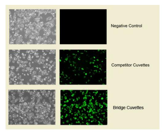
Using the sophisticated **NEPA21 Electro-Kinetic Transfection System**, Bridge Electroporation Cuvettes display lower impedance to electric flow resulting in more power delivered to the sample. Our electroporation cuvettes exhibit an average resistance of 41.5 Ohms with a tight variability of +/-1.5 Ohms. Competitive cuvettes exhibited nearly 30% higher impedance with 4x broader variability.
