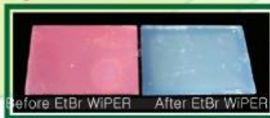
Droplet water containing EtBr was applied to paper towel and sprayed EtBr WIPER to the same paper towel to see the effect of EtBr WIPER.
