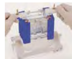
Transfer to casting base and tighten cams
