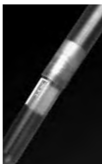
Place sample in CryoTube™, tighten screw cap, cool tube on ice bath, insert the CryoTube into the Nunc CryoFlex
