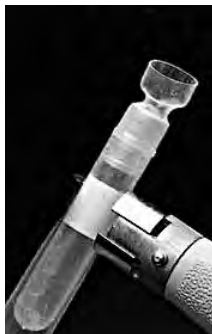
Shrink the Nunc CryoFlex by gentle heating with a heat gun filled with a shrink tube attachment
