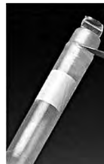
Remove the Nunc CryoFlex by cutting around the screw cap
