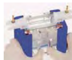
Insert glass plates and slide gates to create efficient seal
