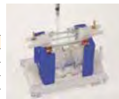
Insert gel solution and comb and allow to polymerise
