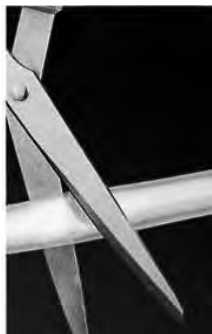
Cut to leave sufficient Nunc CryoFlex at each end of the tube
