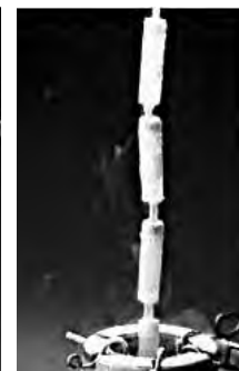
Use Nunc CryoFlex as a cane for liquid nitrogen
