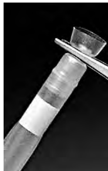
Crimp or squeeze the heated ends. Trim excess tubing and, if desired, melt the crimped ends
