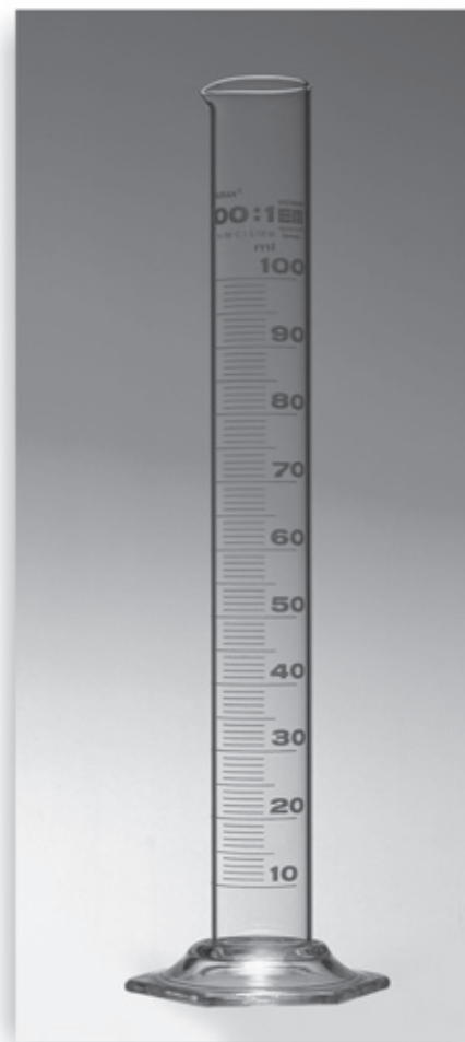
MEASURING CYLINDER, CLASS 'A' EM-TECHCOLOR
