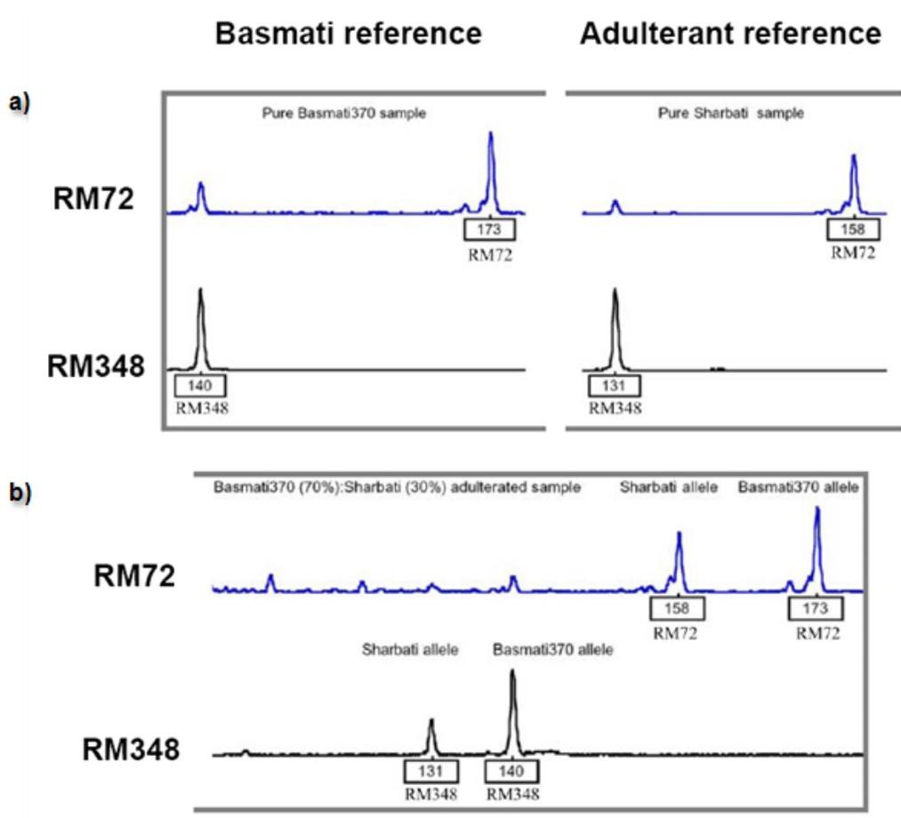
**Figure 2.8 Detection of the adulterant.** a) Electropherogram of amplification of pure Basmati (Basmati370) and pure adulterant (Sharbati) using RM72 and RM348 b) Electropherogram of amplification of adulterated Basmati (Basmati370 adulterated with 30% Sharbati) using RM72 and RM348
