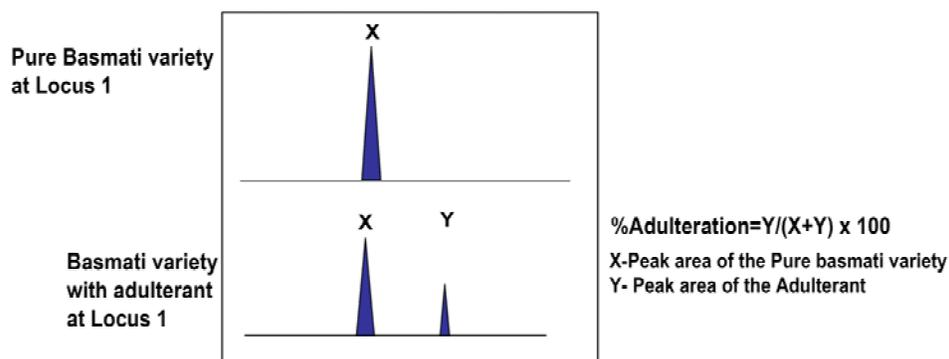
**Figure 2.13 Quantification of the adulterant.** The principle underlying the quantification of the adulterant is that ratio of quantities of the amplicons (ratio of peak area of pure variety and adulterant) is directly proportional to the quantities of competing DNA template in a PCR reaction.
