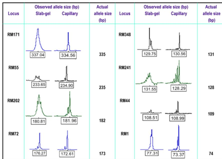
Figure 2.16 Extent of allele size differences between slab-gel and capillary electrophoresis at eight rice microsatellite loci. Each peak represents a single allele, whose size (in bp) is given below the peak. Please see Table 2 for allele size a range; only a representative profile is shown here. The actual allele sizes, determined by bidirectional sequencing, are also provided in the column for comparison.
