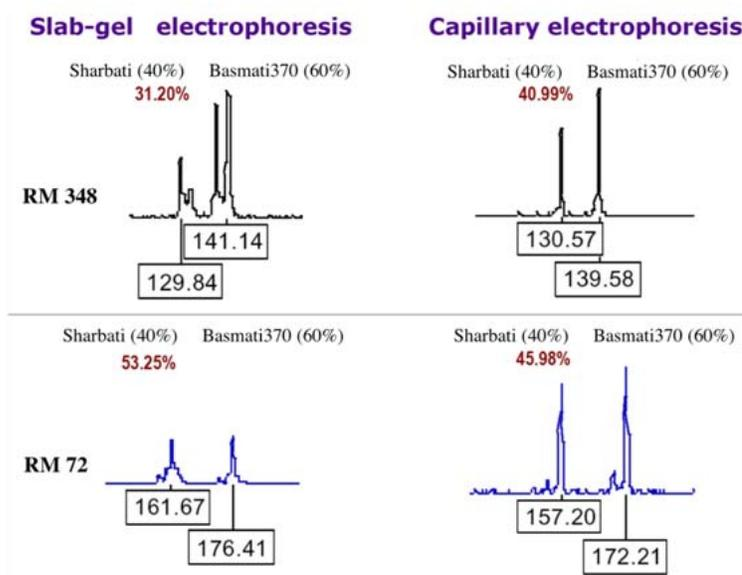
Figure 2.18 Accuracy of slab-gel and capillary electrophoresis techniques in quantification of Basmati rice adulteration. A representative profile of Basmati370 mixed with Sharbati (a common adulterant) in a 60:40 ratio is shown. Adulteration was quantified at two microsatellite loci, RM348 and RM72. Sharbati is detected by the shorter amplicons (left). Peaks are labeled with allele sizes (bp) as determined by Genotyper software; estimated adulteration values (%) are given in bold face.
