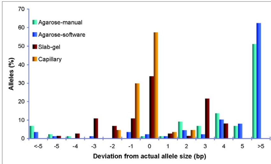
**Figure 2.15 Allele size estimation accuracies of agarose, slab-gel and capillary electrophoresis methods.** Y-axis presents fraction of total alleles (expressed in percentage) showing deviations from the actual allele sizes. X-axis shows the deviation (in bp) of the observed allele sizes from the actual allele sizes obtained by bidirectional sequencing.
